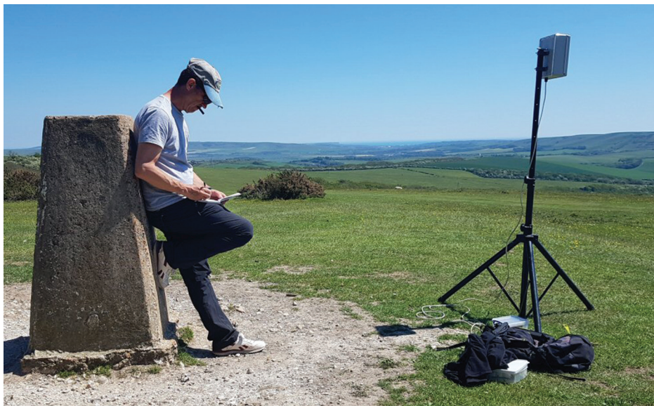
A lovely Spring day for radio experiments on a nearby hilltop (by the way, I am noting transmissions times on a pad while holding the pen lid in my mouth, not smoking a cigar!). The box mounted on the tripod contains the 1mW transmitter and dipole antenna.
