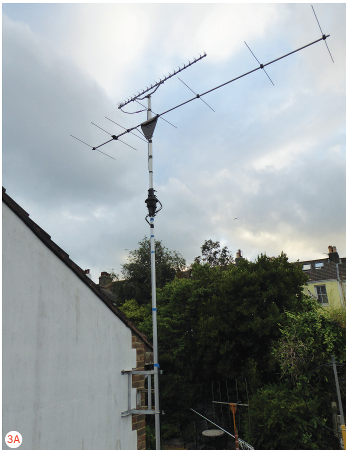
PHOTO 3A-C: 23 element 1296MHz Yagi at home (ca. 60m asl) ii) view of Hollingbury Hill from my house in Brighton (hill top is slightly to the right of centre) and iii) the view back from the top of Hollingbury Hill (178m asl).
