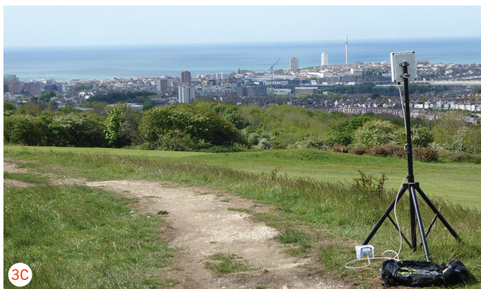
PHOTO 3A-C: 23 element 1296MHz Yagi at home (ca. 60m asl) ii) view of Hollingbury Hill from my house in Brighton (hill top is slightly to the right of centre) and iii) the view back from the top of Hollingbury Hill (178m asl).
